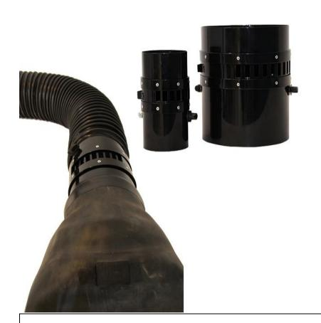
Smart Cool SC is an adapter with a damper, and adjustable grill for adding cooling air. With this function it is possible for the cool air to be added gradually, when extracting high temperature air from i.e. exhaust gas. When the regulation grill is open, it will extract air from the room and mix it with the gas from the vehicle. The product is available in Ø100, Ø125, Ø150 and Ø200 mm.
